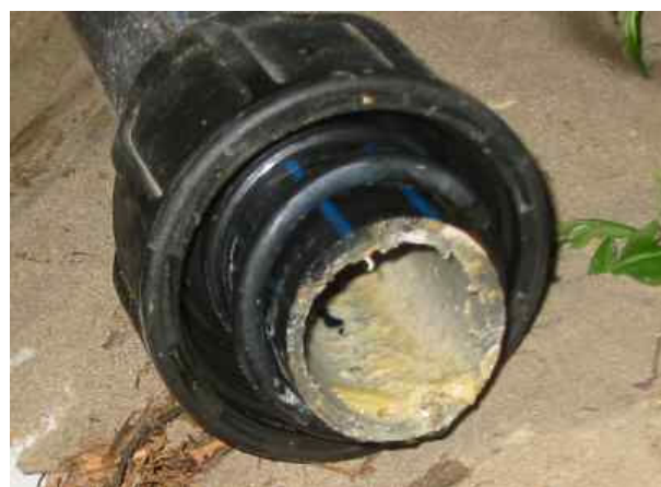
Figure 5 Struvite deposits in the urine collection pipe after 12 months of use.
